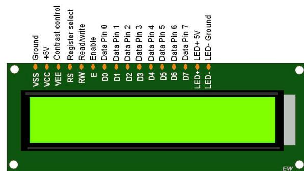
Fig3: Pin Configuration Of LCD
