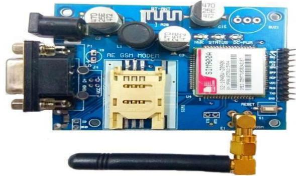
Fig 7: GSM (SIM 900) Module
