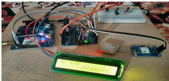
Fig 12: Prototype of Soldier Health and Position Tracking System
