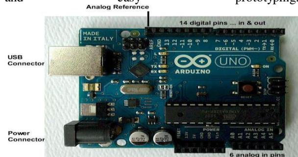
Fig 2: Arduino Development Board
